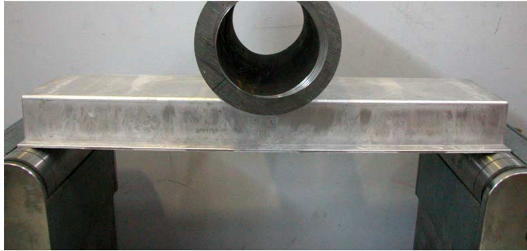
Fig. 7. Test set-up for 3-point bending, load case (n).
