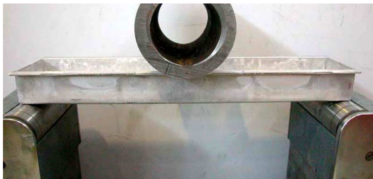
Fig. 8. Test set-up for 3-point bending, load case (u).
